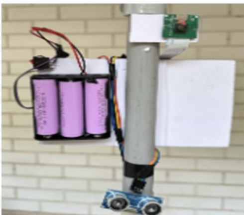
Fig.4. Pi-camera, Battery, Ultrasonic sensor
