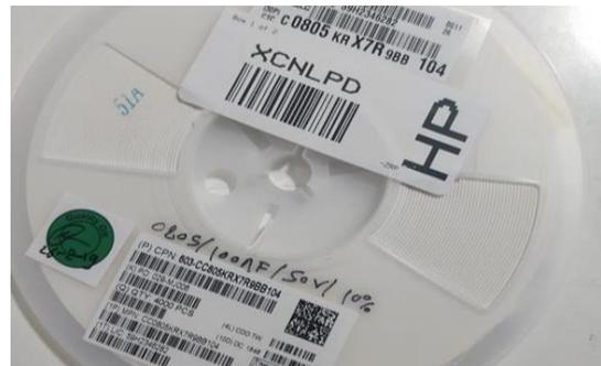
Fig.12. Components in Reel Form
