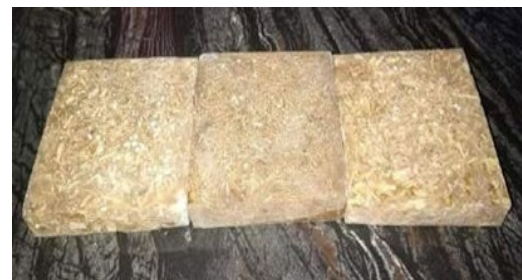
Fig.11. Image of the Coconana Fiberboard after subjected to drop test
