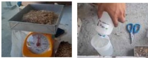
Fig.5. Weighing Raw Materials and Mixing Epoxy Resin and Hardener
