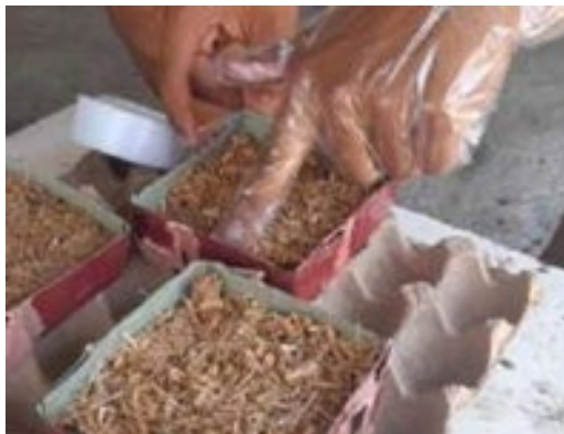
Fig.6. Putting the fibers into the molder
