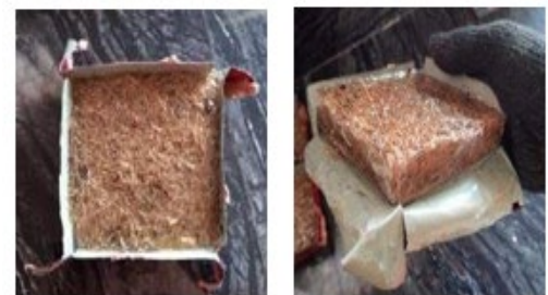
Fig.9. Removing of fiberboard from the molder
