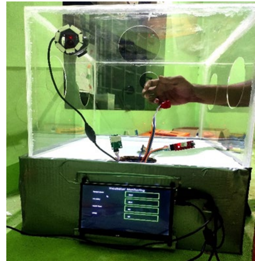
Fig.9. Image depicting the positioning of the LCD Touchscreen
