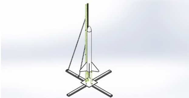
Fig. 1. Portable launch pad 3D model
