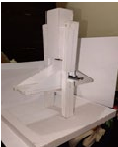
Fig. 3. Tipping bucket rain gauge
