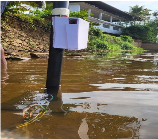
Fig. 9. Measuring distance using ultrasonic sensor at 64cm
