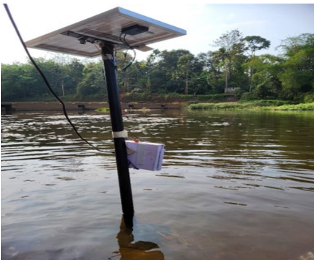
Fig. 11. Measuring distance using ultrasonic sensor 75cm
