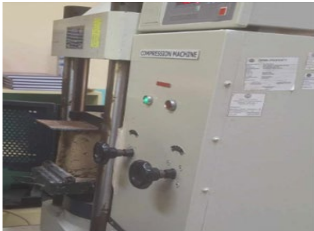
Fig. 3. Compression strength test on the specimen
