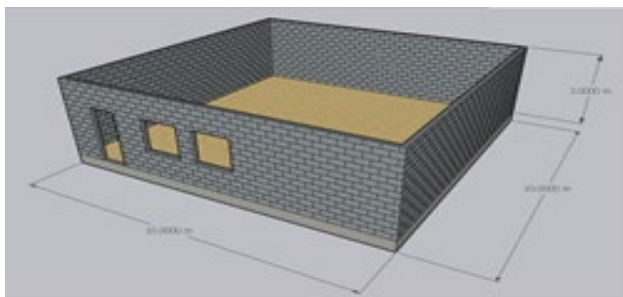
Fig. 9. 120sq 2 wall area using concrete hollow block
