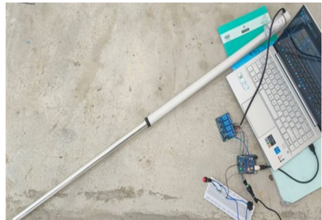
Fig. 11. Motor controlling unit
