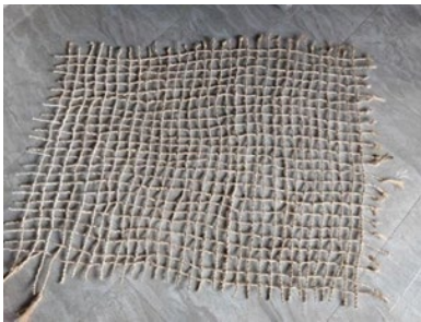
Fig. 5. Finished product latex-coated banaca geotextile net
