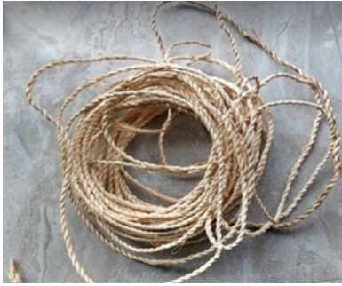
Fig. 4. Finished product latex-coated banaca geotextile rope
