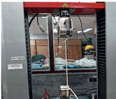
Fig. 6. Twined fiber tensile strength test (ASTM D2256)
