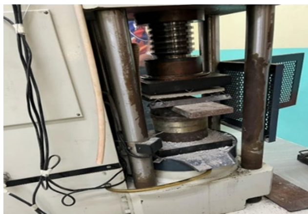
Fig. 7. Flexural strength test using third point loading
