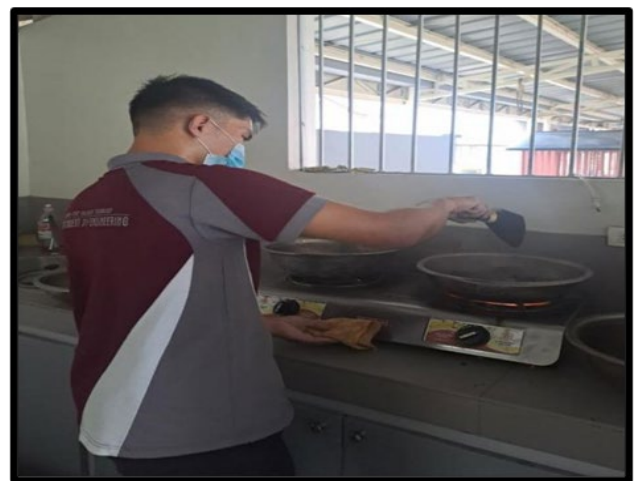
Fig. 7. Preparation of Paving Asphalt/Mixing of Materials
