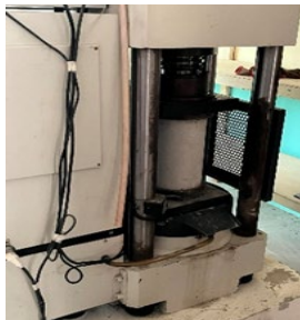
Fig. 7. Compressive testing for cylinder
