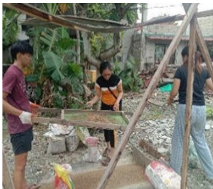
Fig. 4. Sieving and grading of pulverized glass
