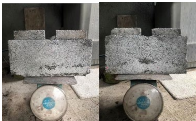
Fig. 15. Mass result of CLB 1 and 2, respectively
