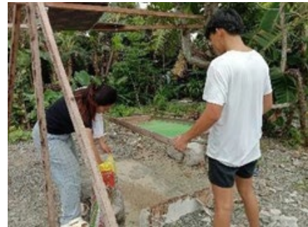
Fig. 6. Sieving and grading of pulverized glass
