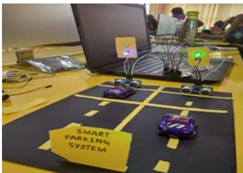
Fig.5. Hardware part where the ultrasonic sensors and led lights
