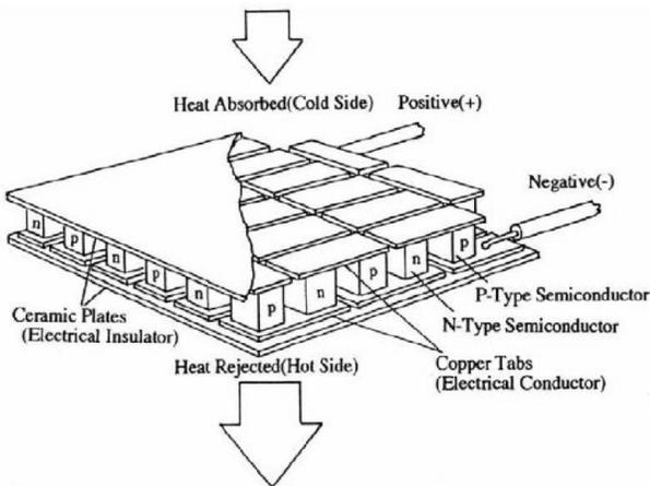
Fig.2. Construction of Thermoelectric Module [3]
