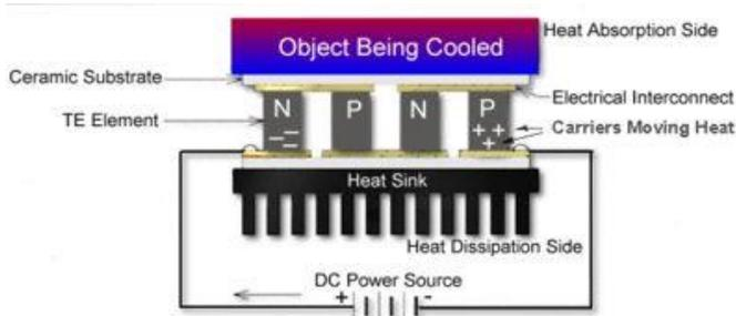
Fig.3. Schematic Diagram of Thermoelectric Cooler [28]
