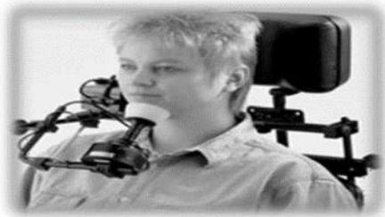
Fig.2.4. Power wheel chair chin-operated force sensing joystick
