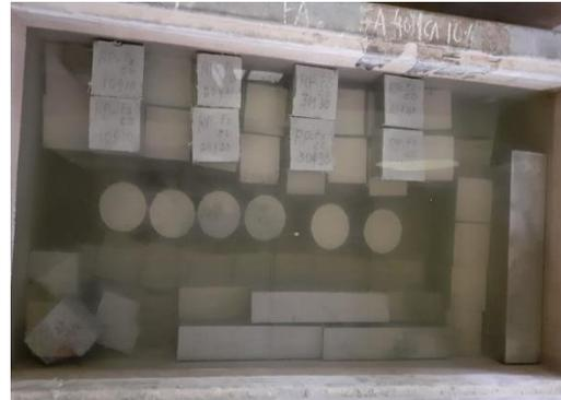
Fig.5. Curing of specimens in curing tank
