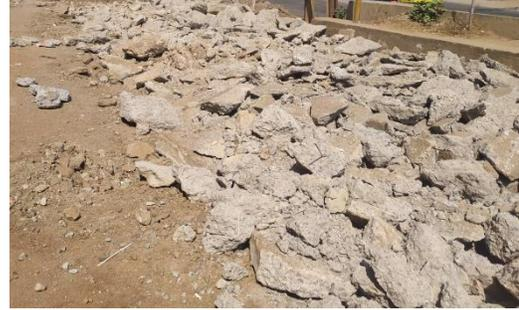
Fig.2. Raw material of C & D waste from Road concrete
