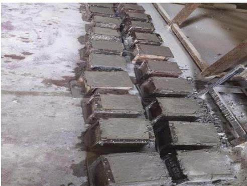
Fig.4. sample of cube Casting
