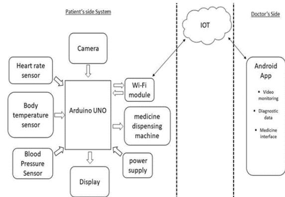
Fig.1. Block diagram of the health companion system.
