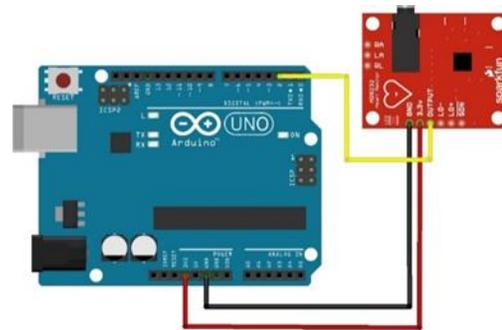
Fig.2. Interfacing of heart beat sensor with Arduino.
