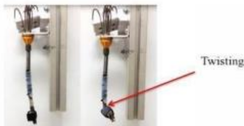
Fig.9. Twisting of spring due to gravity/load.
