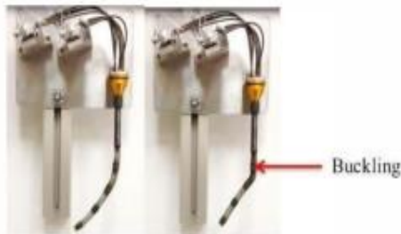
Fig.8. Joint buckling due to coupling of springs.
