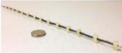
Fig.11. Springs and spacer arrangement using nitinol.
