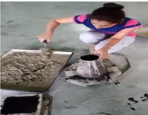
Fig.3. Concrete mix for M-30 (Slump Cone Test of concrete)
