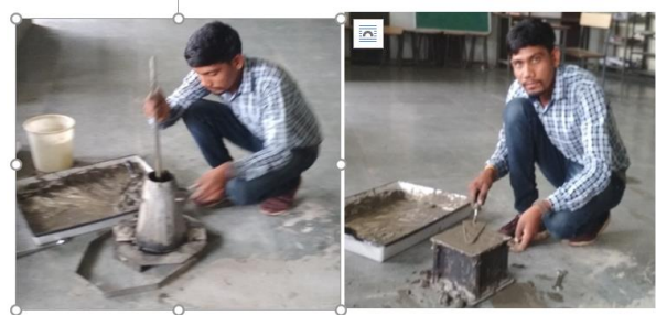
Fig.2. Concrete Mix for M-40 (Slump Cone Test of Concrete)
