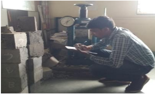
Fig.3. Testing of Cubes in Laboratory On Compressive Testing Machine
