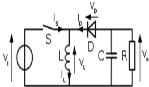
Fig.10. Schematic of a buck–boost converter.
