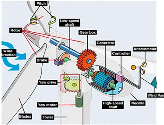
Fig.7. Over view of wind turbine
