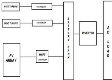
Fig.2. Circuit diagram for solar power
