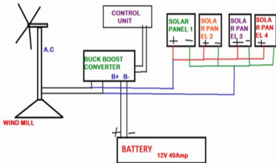
Fig.8. Block diagram of a PV/wind hybrid energy system
