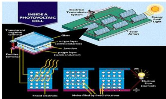
Fig.3. Overview of solar system equipment's
