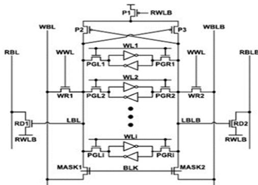
Fig.7. Proposed SRAM architecture that stores  $i$  bits in one block.
