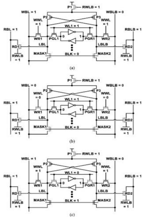
Fig.9. (a) Selected, (b) row half-selected, and (c) column half-selected blocks of proposed SRAM architecture during write operation.
