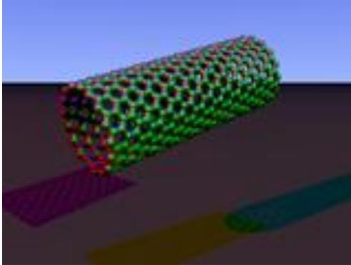
Fig.3. Structure of a SWCNT.
