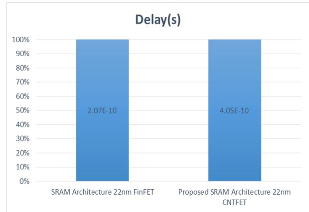
Fig.13. Comparison of delay of 22nm FinFET SRAM architecture with 22nm CNTFET SRAM architecture.
