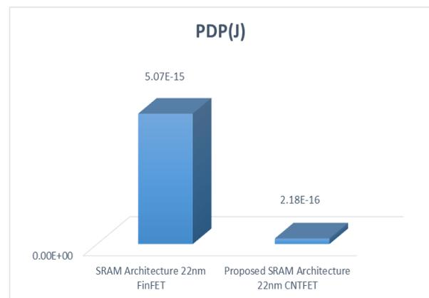
Fig.14. Comparison of power delay product (PDP) of 22nm FinFET SRAM architecture with 22nm CNTFET SRAM architecture.
