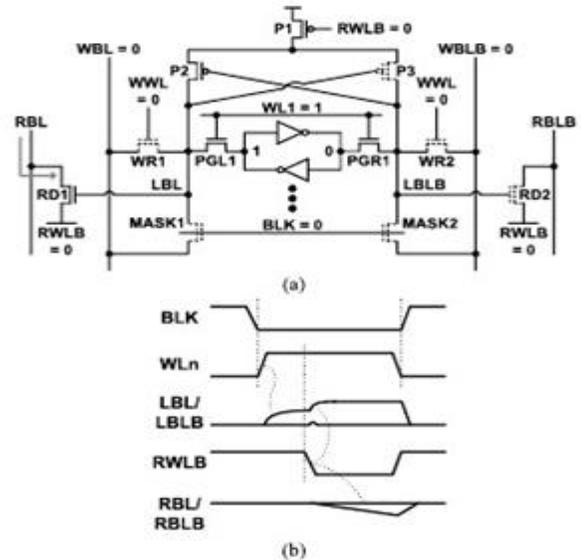
Fig.8. (a) Read operation and (b) read Operational waveform of proposed SRAM architecture.
