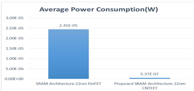
Fig.11. Comparison of average power of 22nm FinFET SRAM architecture with 22nm CNTFET SRAM architecture
