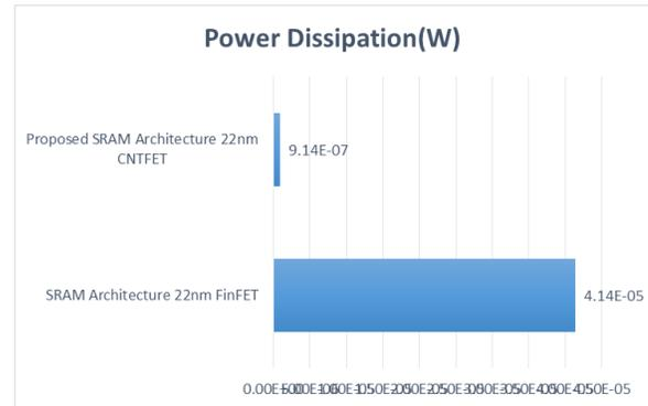
Fig.12. Comparison of power dissipation of 22nm FinFET SRAM architecture with 22nm CNTFET SRAM architecture.
