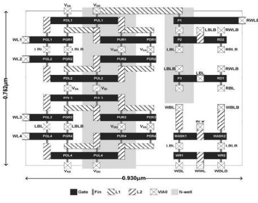
Fig.10. Layout of the proposed SRAM architecture based on the 22-nm CNTFET technology.
