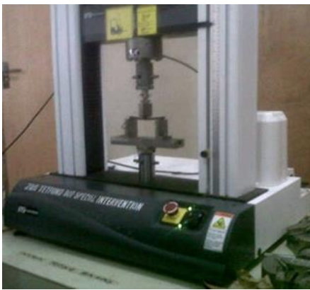
Fig.4. Composite under Flexural Testing Using Instron Machine.
