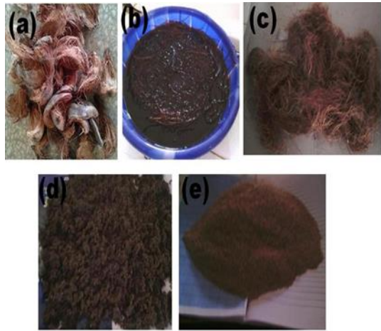
Fig.1. Coir Fibre And Wood Dust Processing, Showing (A) Coir Husk (B) Coir Fibre In 5% Naoh Solution (C) The Oven Dried Fibre (D) The Oven Dried Wood Dust (E) The Sieved Wood Dust.
