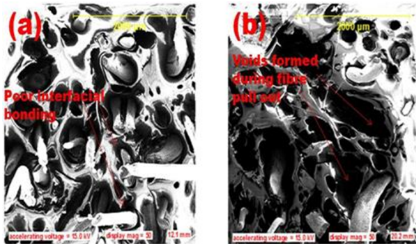
Figure.6. SEM Micrographs of Composites, Showing (A) C10 and (B) C10S1.
