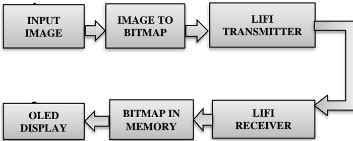
Fig 5: Block Diagram of Image Communication
