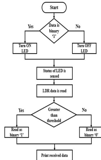
Fig.2. Flowchart of Li-Fi communication
