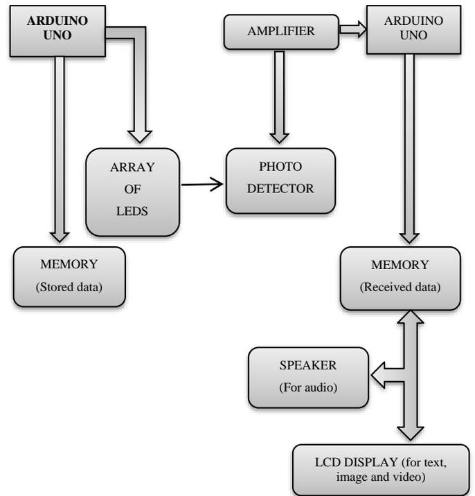
Fig 1: Block diagram of proposed Li-Fi Module.
