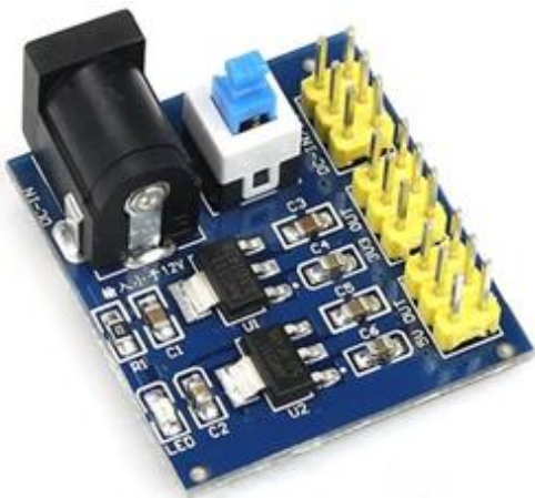
Fig.10. Power Supply Module
