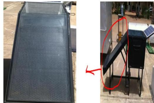
Fig. 1.a Normal Collector 1.b Solar dryer
