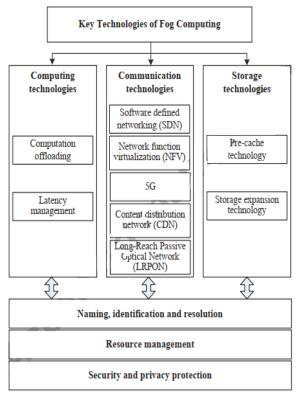
Fig.3. the key technologies of fog computing [18].
