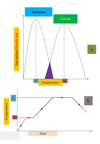
Fig.2. To make a glass-ceramic, glass crystallization used. (a) Temperature affects nucleation and growth rates, with minimal overlap. (b) a two-stage heat treatment
