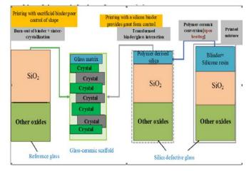
Fig.4.Glass-ceramic processing schemes: traditional devitrification (left) vs heat treatment of silicone/silica-defective glass mixes (right) [48]
