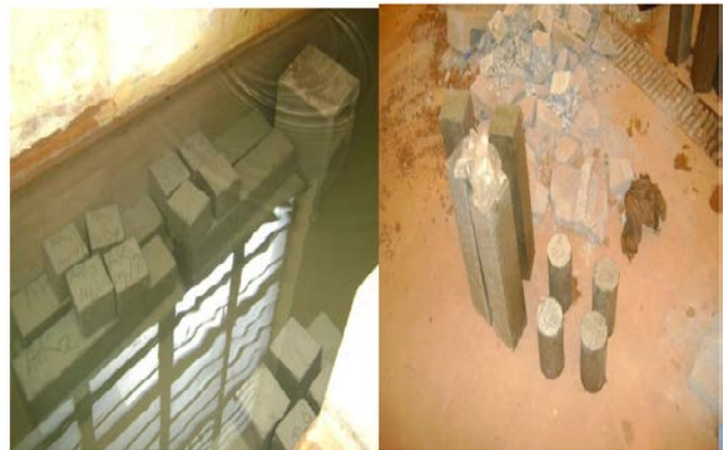
Fig.3. (a) Test Samples in the curing Tank (b) Some of the Test Samples after removal from the curing Tank
