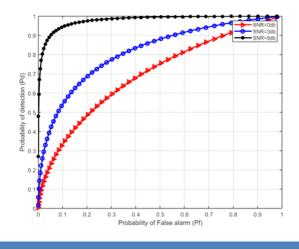
shows the probability of detection under various SNR values. The time bandwidth product u is kept 10 and threshold to 20. Fig. shows the Receiver operating characteristic (ROC) between probability of detection vs. probability of false alarm with varying SNR. It is noted that when less noise is observed on the channel i.e., when SNR is high, detection probability is better as it indicates the presence of primary user signal.
