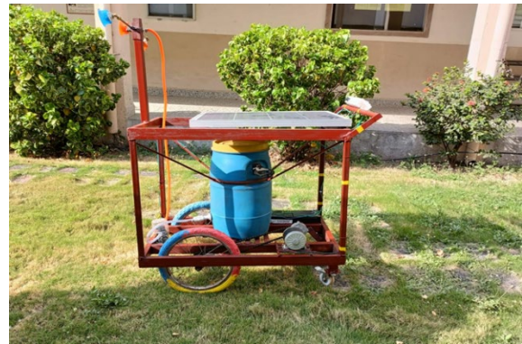
Fig.6. Realtime images of automatic solar sprayer
