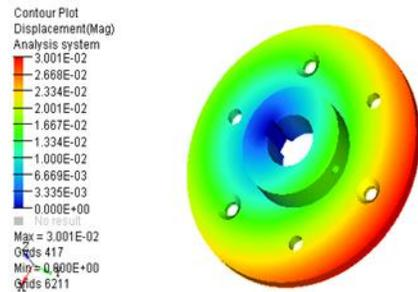
Fig.13. Total Deformation in Flange
