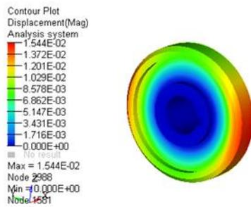
Fig.9. Total Deformation in Rotor
