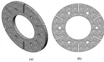
Fig. 3 (a) Isometric View of Armature (b) Front View of Armature
