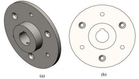
Fig. 5 (a) Isometric View of Flange (b) Front View of Flange
