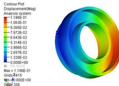
Fig.7. Total Displacement in Stator
