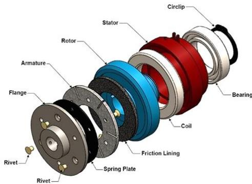
Fig. 16. Exploded View of the Clutch Assembly
