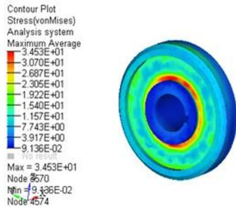
Fig.8. Total Stress in Rotor
