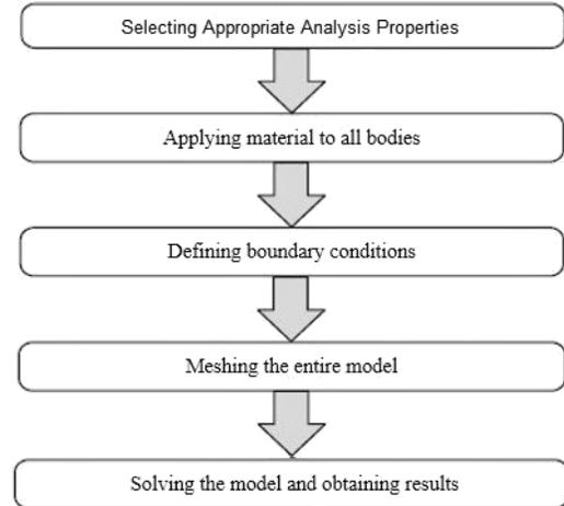
Fig. 17. Steps followed for the Magneto-static Analysis
