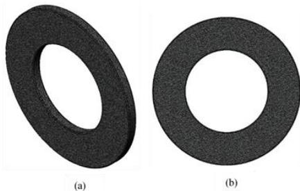
Fig. 4 (a) Isometric View of Friction Lining (b) Front View of Friction Lining
