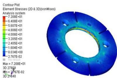
Fig.10. Total Stress in Armature
