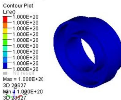
Fig.14. Fatigue Analysis of Stator
