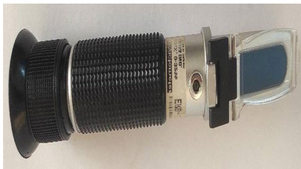
Fig.3. Measuring TSS (Total Suspended Solids) On Refractometer
