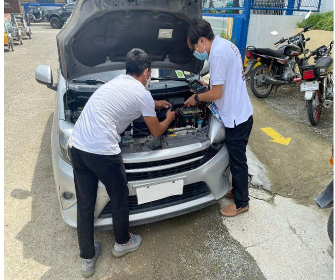
Fig.1. The actual installation of the developed Immobilizer Compact System (ICS) using the GPS-GSM module
