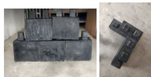
Figure 16: Interlocking of Lego-Inspired Blocks
