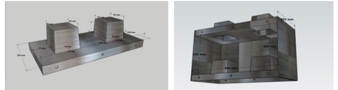
Fig. 3&4: Dimension of the top & body portion of the mold
