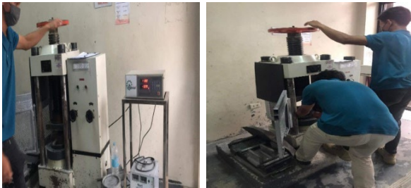
Figure 20: Actual photos of UTM for Flexural Strength in Unified Geotest Laboratory
