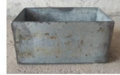
Figure 18: Mold for flexural test specimen with a dimension of 200mm x 120mm x 100mm
