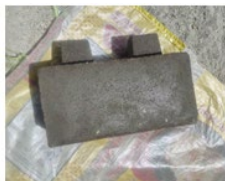
Figure 15: 400 mm x 200 mm x 200 mm sample block
