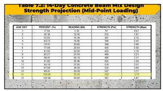
Flexural strength must not be less than 4.5MPa when tested by the mid-point method at fourteen (14) days in accordance with AASHTO T177
