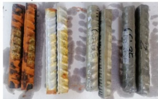
Figure 3: Bio-based Coated Reinforcing Steel Bars (65:35)
