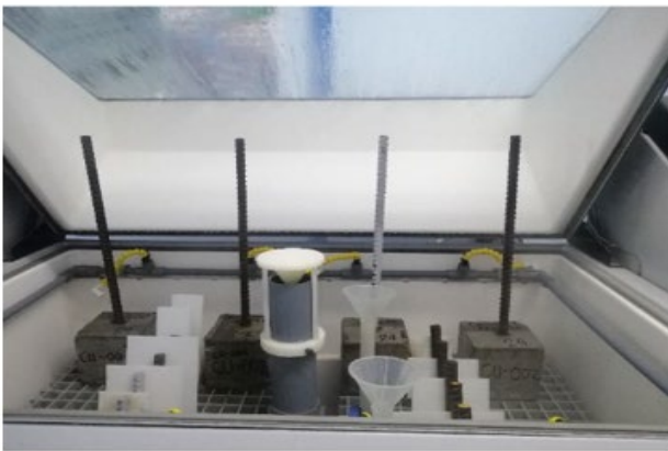
Figure 2: Set-up of Reinforced concrete samples in the corrosion chamber
