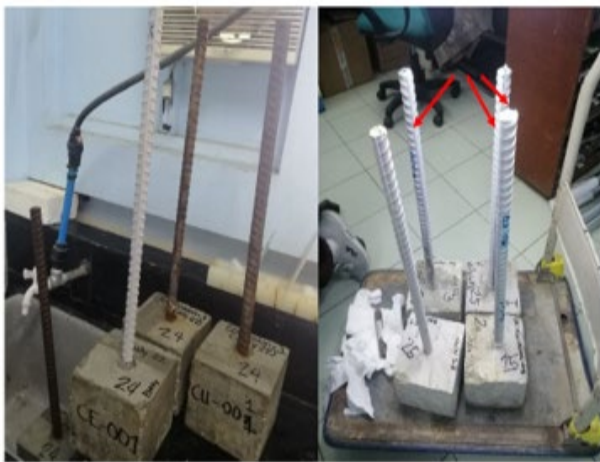
Figure 5: Rust Formation in the Reinforced Concrete Samples after the Salt Spray Test
