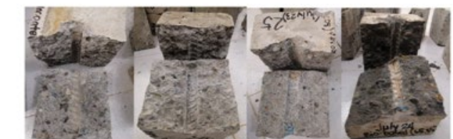
Figure 6: Concrete Splitting with (a) Uncoated Steel Bars; (b) Epoxy Coated Steel Bars; (c) Bio-based Coated Steel Bars, 50:50; (d), 65:35
