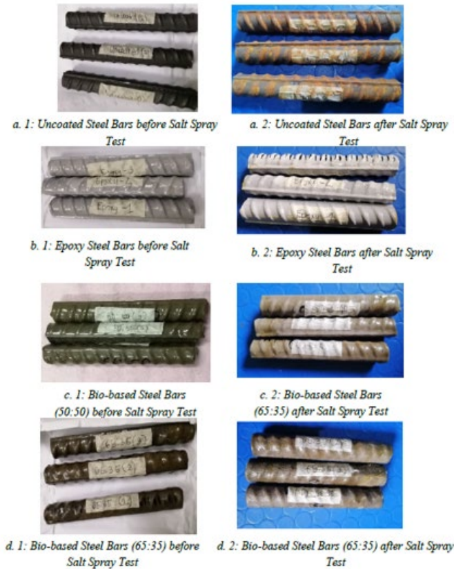
Figure 4: Results of the reinforced concrete samples subjected to Salt Spray Test
