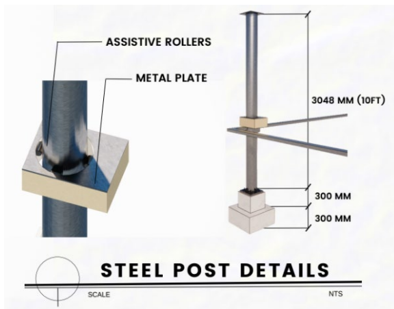
Fig.16. Steel Post Details
