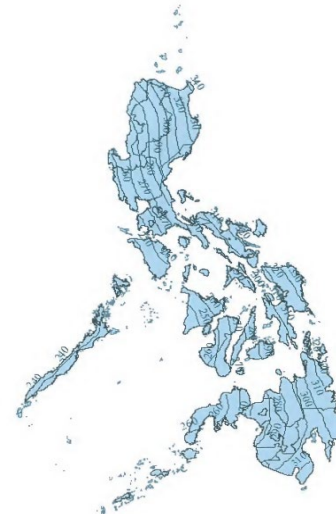
Fig. 2.1-B Basic Wind Speeds for Occupancy Category III, IV and V Buildings and Other Structures from Figure 207A.5-1B of NSCP 2015
