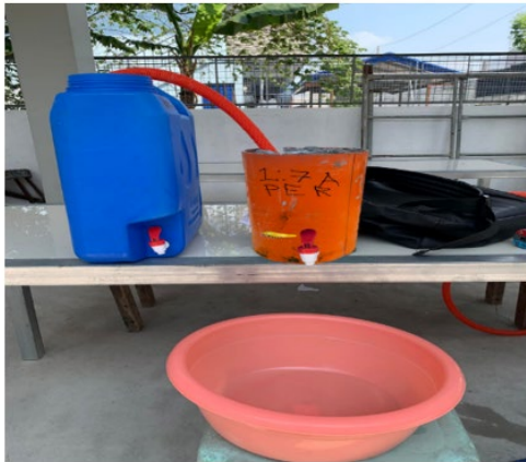
Fig.6. Constant Head Permeability Test Set-up
