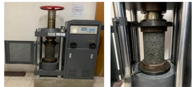
Fig.5. Compressive Strength Test Set-up
