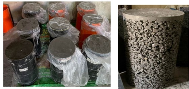
Fig.4. Pervious Concrete Specimen
