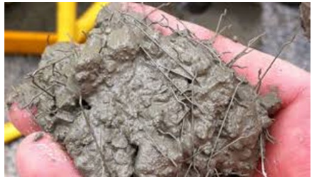
Fig.1. Steel Fiber Reinforced Concrete
